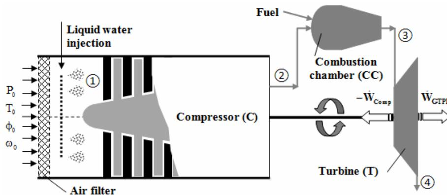
Fig. 1 – Physical configuration of a GTTP employing the "fog cooling" technology with complete vaporization before the admission into the compressor of the liquid water sprayed into the intake.
