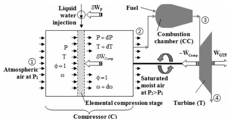
Fig. 3 – Adjacent elemental compression stages within the internal volume of the GTPP’s axial compressor.
