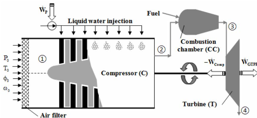
Fig. 2 – Physical configuration of a GTPP employing the “inter-stage water spraying” technology.
