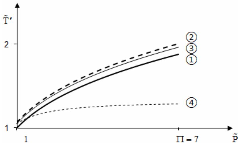
Fig. 4 – Temperature variation of the compressed moist air when using different types of temperature control.
