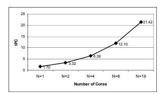
Fig. 10 - The IPC of SLVP-based architectures.
