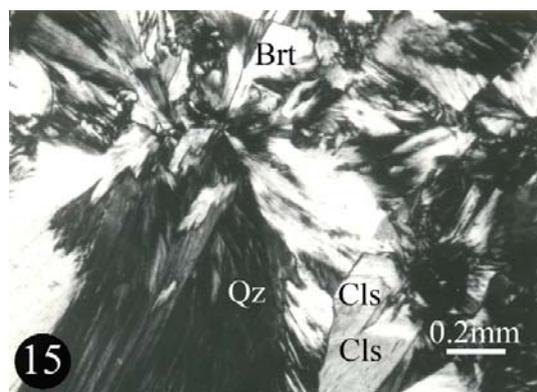
Fig. 15 – Fibro-radial quartz (“quartzine”) partly substituting barite (Brt) and celestine (Cls). N+.
