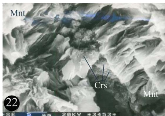
Fig. 22 – SEM: Vermicular structures of Na-smectite (Mnt) and cristobalite (Crs) (sample 7).
