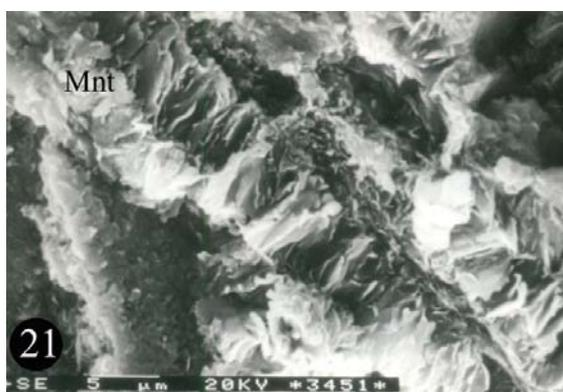
Fig. 21 – SEM: Vermicular structures of Na-smectite (Mnt) (sample 5).
