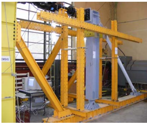
Fig. 9 – Experimental test setup for brace tests.
