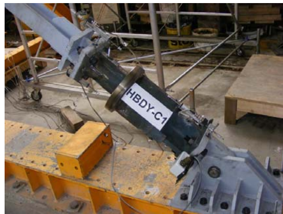
Fig. 10 – Experimental test setup for brace with damper assembly tests.
