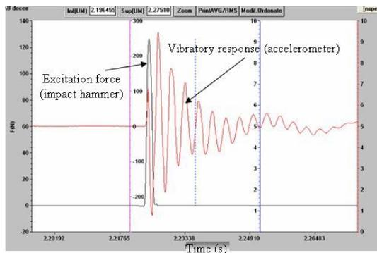
Fig. 9 – Experimental recordings (bar 2 – Variant 1).
