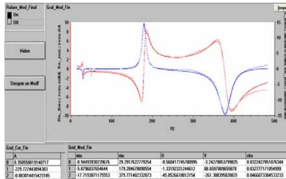
Fig. 4 – The final panel of modal parameters (model 2).
