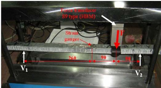
Fig. 5 – The bending loading scheme and device (model 1).
