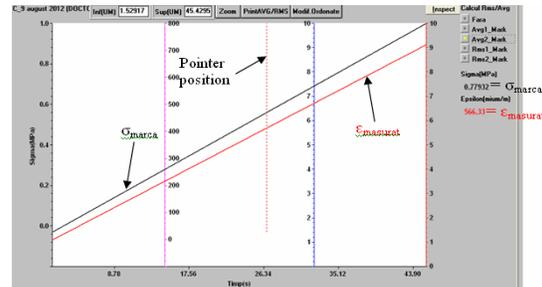
Fig. 6 – The stress and strain at a chosen point from the experimental data.
