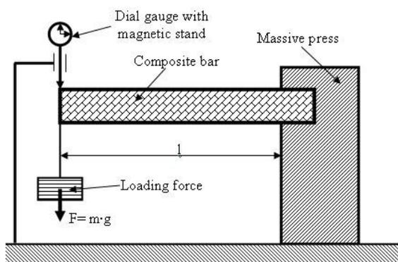
Fig. 13 – Experimental assemblage.
