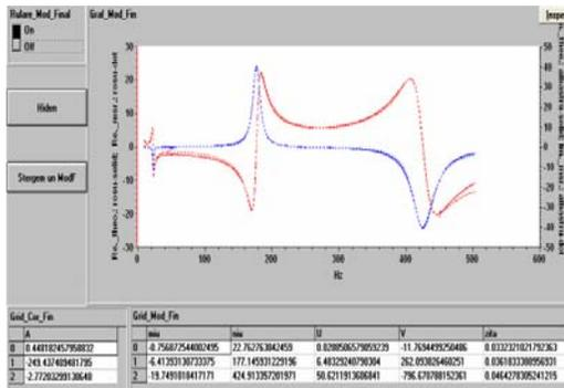
Fig. 3 – The final panel of modal parameters (model 1).
