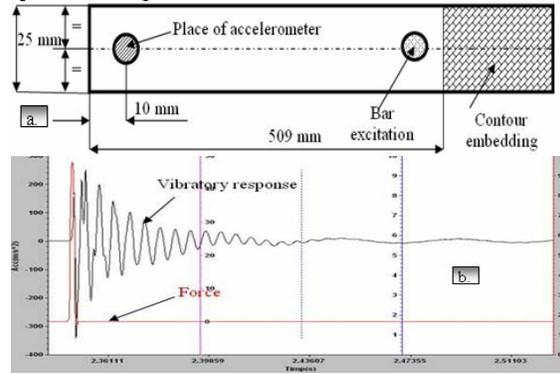
Fig. 2 – a. The experimental scheme; b. experimental recordings (model 1).
