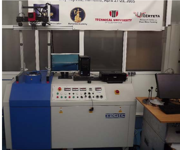
Fig. 5 – Erichsen testing machine (model 142–20) and ARAMIS strain-measurement system used for the experimental determination of the forming limit curve.
