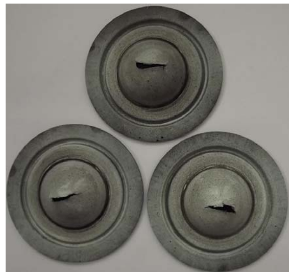
Fig. 7 – Hydraulic bulge test samples of Bondal sheet.
