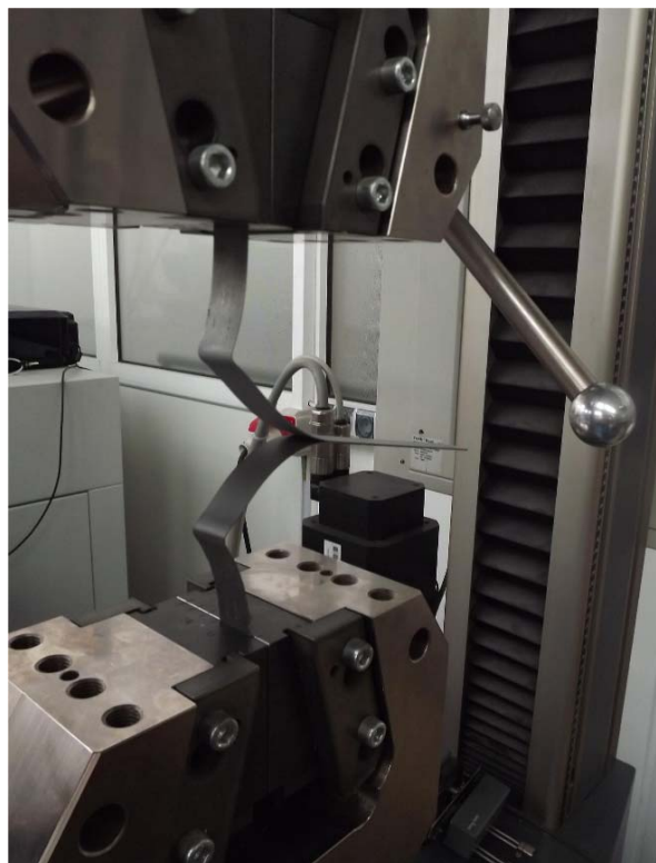
Fig. 9 – The T-peel test performed on a Bondal sandwich sheet.
