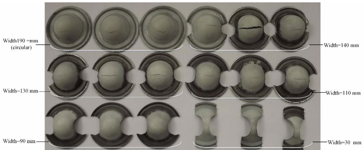
Fig. 4 – The six Nakazima test samples with three repetitions.
