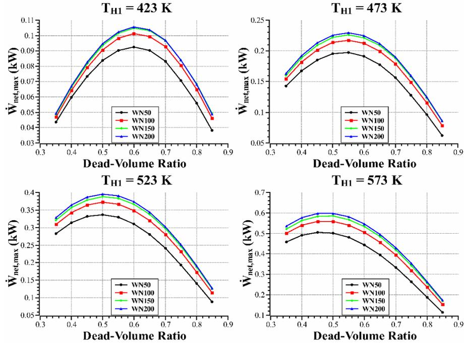
Fig. 1 – Network output versus dead-volume ratio at the four different source temperatures.
