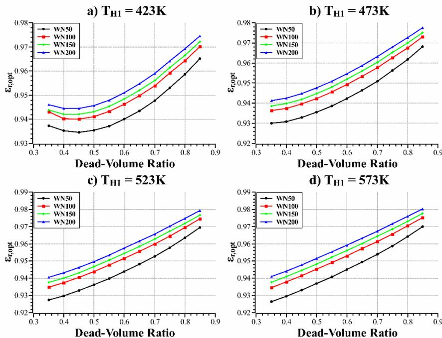
Fig. 4 – Regenerator effectiveness versus dead-volume ratio at the four different source temperatures.
