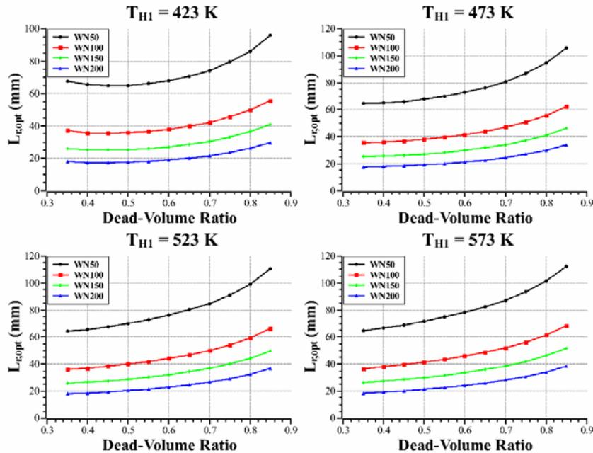
Fig. 3 – Regenerator length versus dead-volume ratio at the four different source temperatures.
