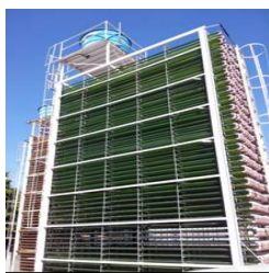
Fig. 1 – Left: compact tubular photobioreactor at Federal University of Paraná, Curitiba, Brazil, and right: branching used for the proposed mass flow rate sensor.
