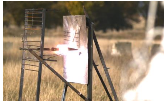
Fig. 5 – The beginning of the jet formation at t = 2.1 ms after the round passed between the bars
