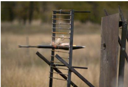
Fig. 6 – PG-7 round hits a bar.
