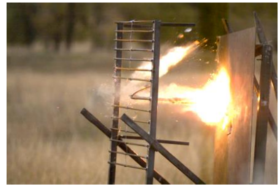
Fig. 7 – The explosive transformation observed at t = 2.6 ms after the impact between the round and the witness plate.
