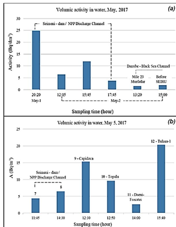
Fig. 2 – HTO activity concentration in water taken at different hours, May 2017:
