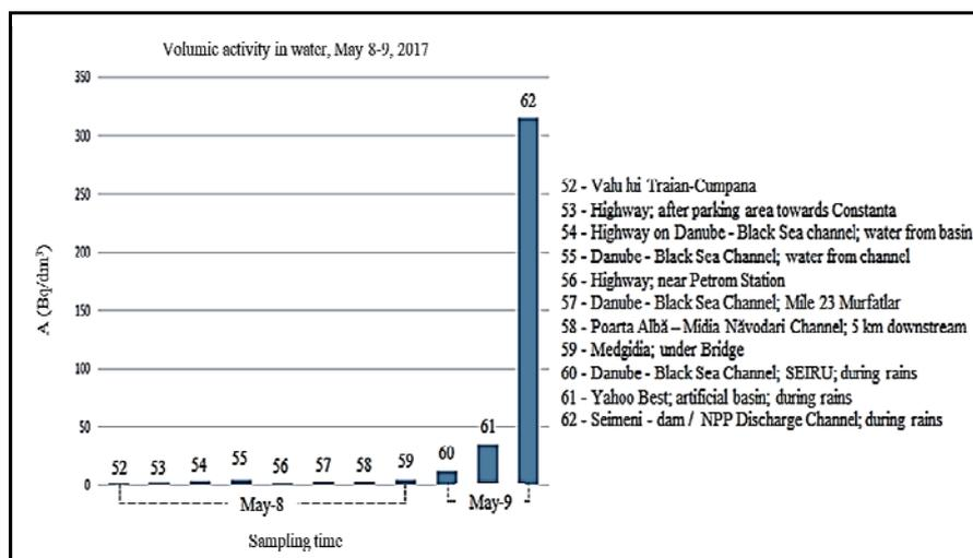
Fig. 4 – HTO activity concentration in water, May 8-9, 2017; logistic sampling points 52 to 62.
