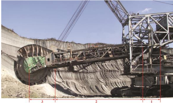
Fig. 2 – The sections of the bucket wheel's boom.
