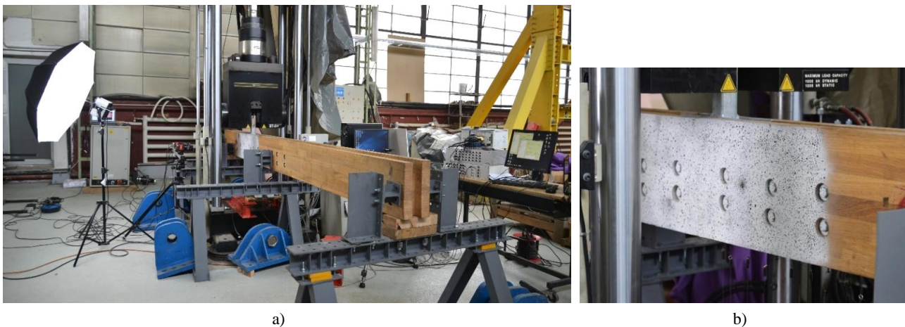
Fig. 8 – View from laboratory: a) test setup and specimen ready for testing; b) surface preparation for VIC-3D measurements.
