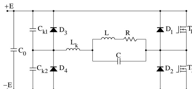
Fig. 1 – Electrical scheme of the transistor inverter.
