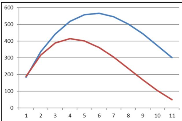
Fig. 3 – Graphical dependency of inverter currents (axes abscise is  $\theta$  [rad],  $\theta = 0.2 i$ ,  $i = 1, \dots, 11$  and axes ordinate current  $i_r$  in [A]).
