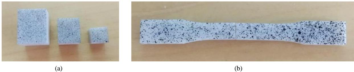
Fig. 3 – Printed specimens for traction and compression prepared for DIC testing: (a) compression; (b) traction.
