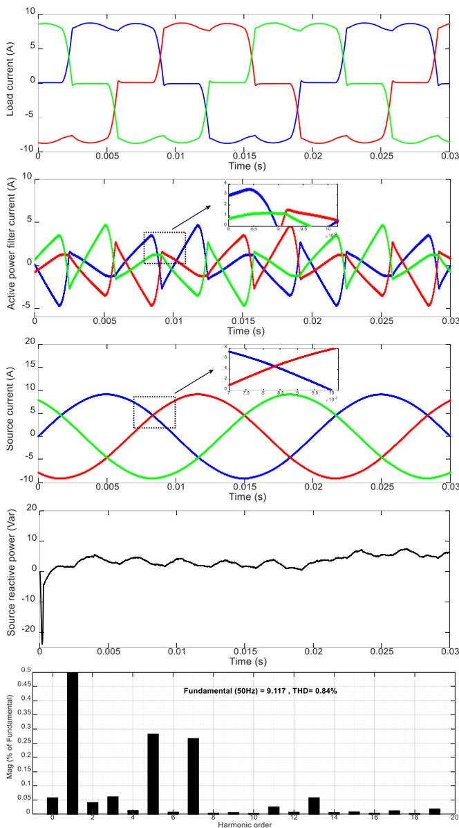
Fig. 9 – Power system responses with presence of ASHC-MLI based SHAPF: a) load current; b) SHAPF current; c) source current; d) source reactive power; e) FFT spectrum of the compensated current.
