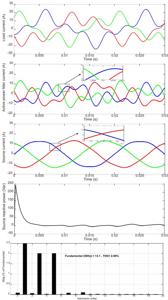
Fig. 11 – Power system responses with presence of ASHC-MLI based SHAPF: a) load current; b) SHAPF current; c) source current; d) source reactive power; e) FFT spectrum of the compensated current.
