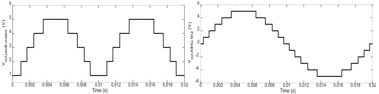
Fig. 4 – Output voltages of proposed multilevel inverter considering 11-level state.
