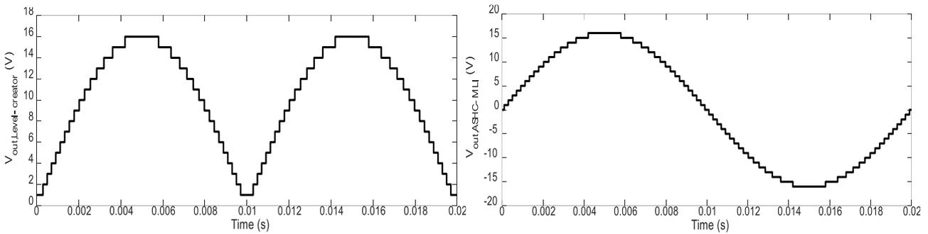
Fig. 5 – Output voltages of proposed multilevel inverter considering 33-level state.
