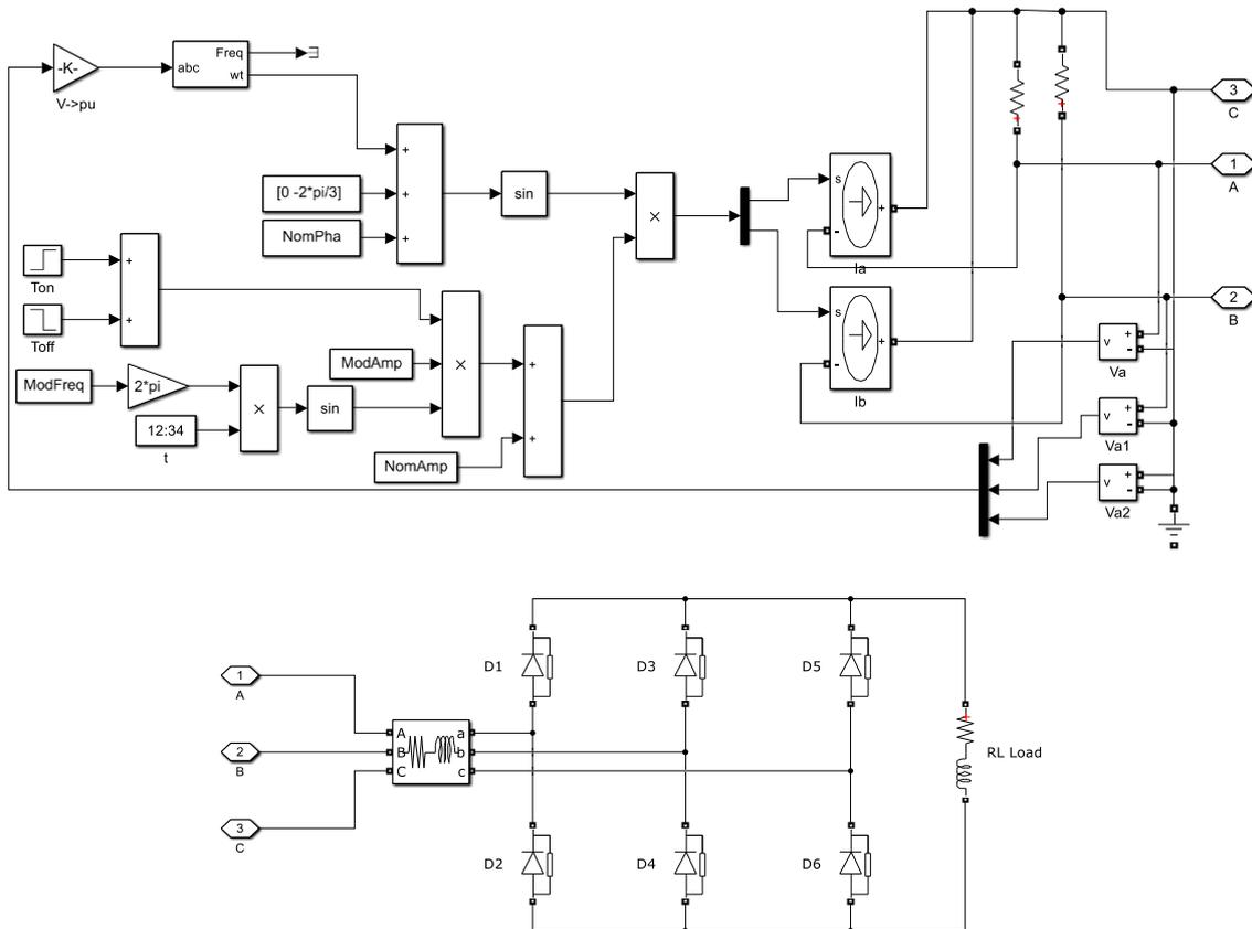
Fig. 8 – The furnace and rectifier load models.
