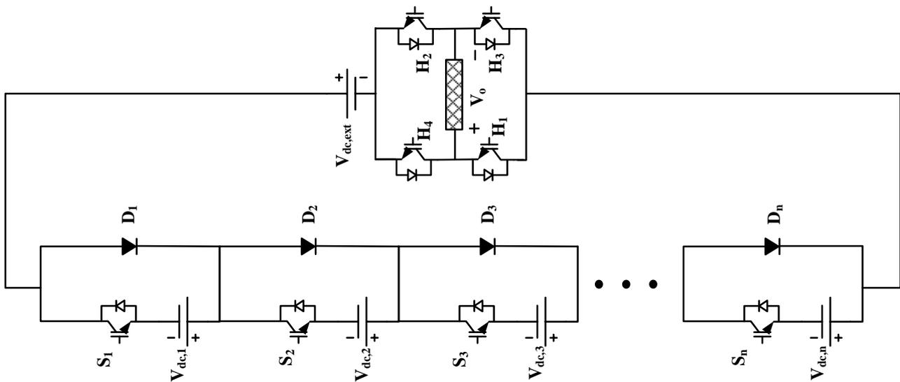
Fig. 3 – General structure of asymmetric/symmetric half-cascaded multilevel inverter.
