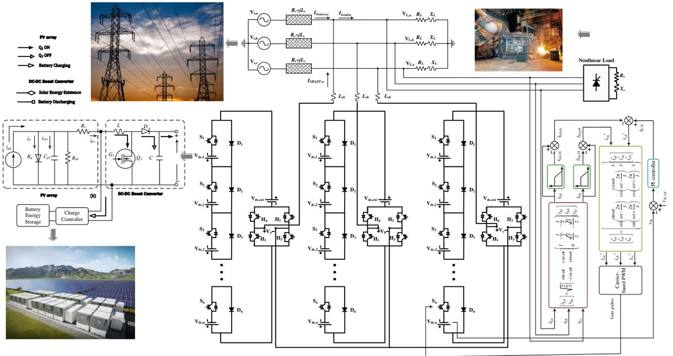
Fig. 1 – The power system with presence of proposed ASHC-MLI based SHAPF.
