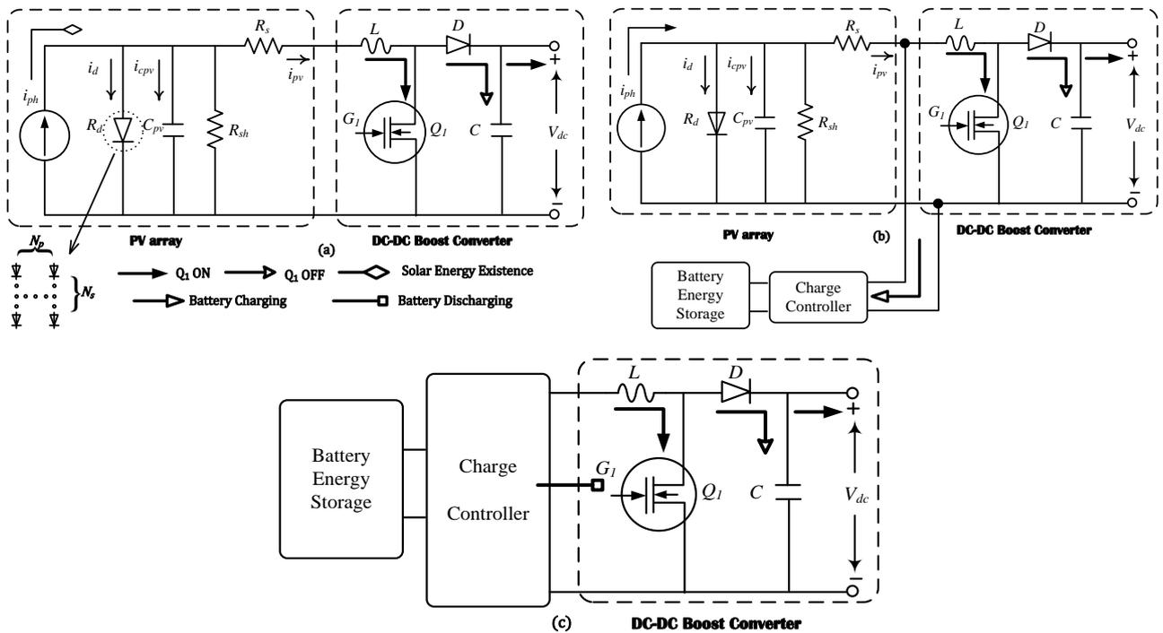
Fig. 2 – The PV current flow under three different operation conditions.
