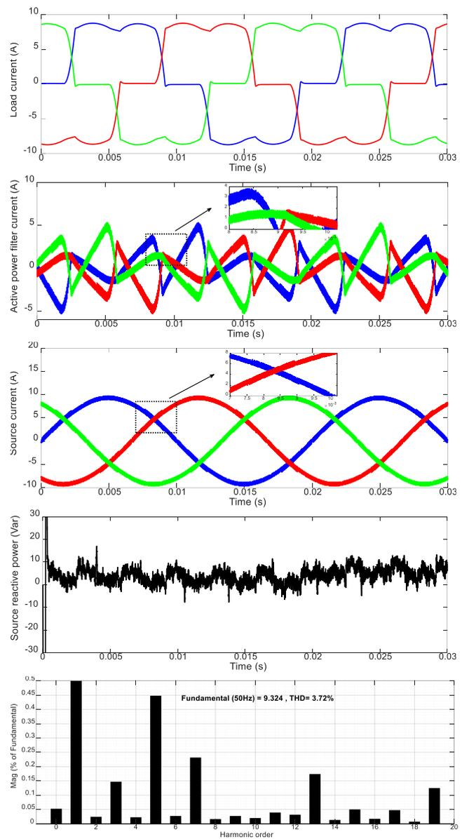
Fig. 10 – Power system responses with presence of conventional inverter based SHAPF: a) load current; b) SHAPF current; c) source current; d) source reactive power; e) FFT spectrum of the compensated current
