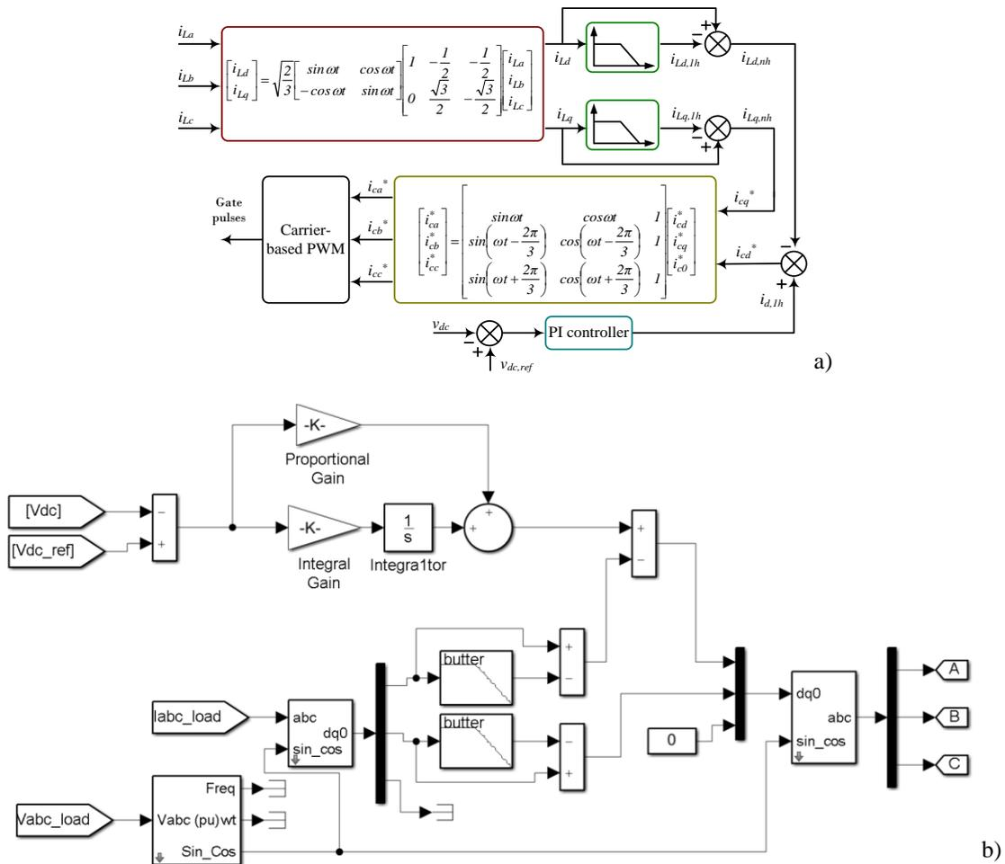
Fig. 7 – The general gate pulse generation strategy: a) block diagram model; b) MATLAB Simulink model.
