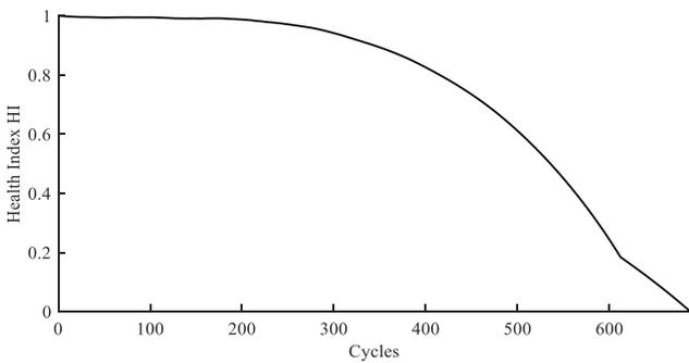
Fig. 6 – Weighted Hellinger distance curve of a test sample.
