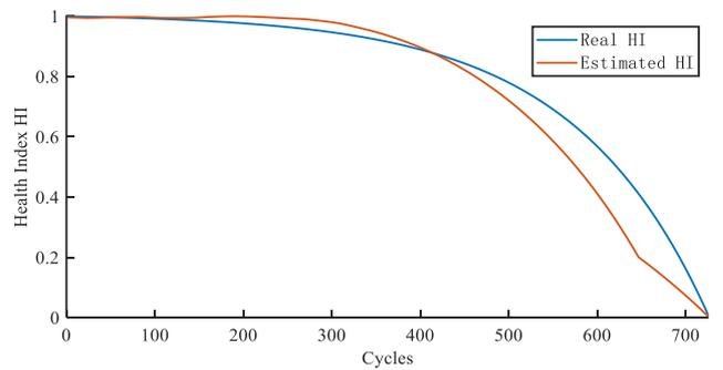
Fig. 7 – The estimated HI and the real HI in a test sample.
