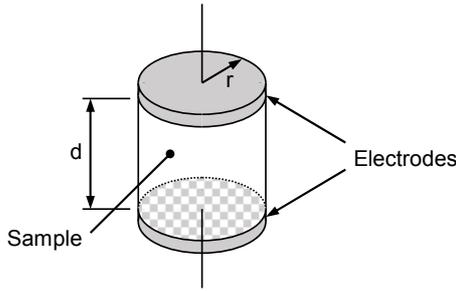
Figure 2. Electrode and sample geometry.
