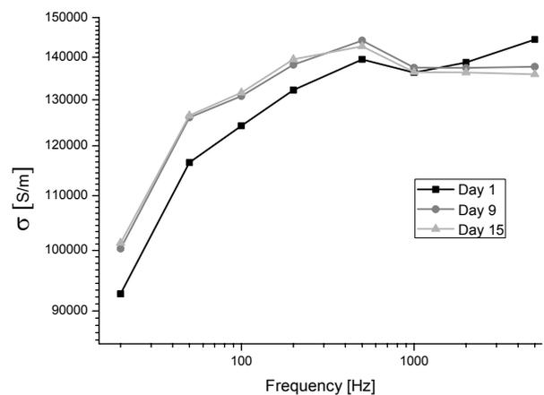
Figure 8. Conductivity evolution (transverse section).
